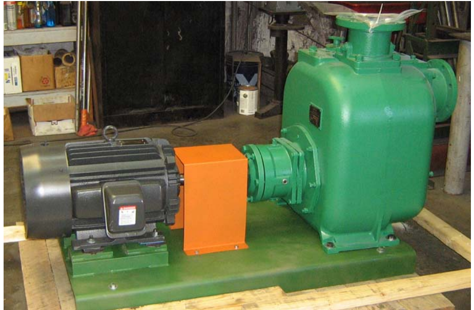
Cornell's new self-primer pictured above was frame mounted at MECO's Simpsonville, SC shop.
