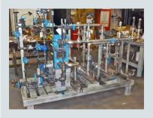
A long-time, repeat customer needed to install a steam heating system on short notice in order to maintain jacketed pipe temperatures for a new manufacturing line. MECO designed and fabricated the system skid, allowing for access and final footprint constraints. This skid contained a Tranter heat exchanger, Corcoran
